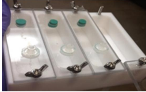
Figure 2.2. Four-chamber polycarbonate drip-flow reactor with septa and filter units used for growth of P.ADP biofilms. 5,9
